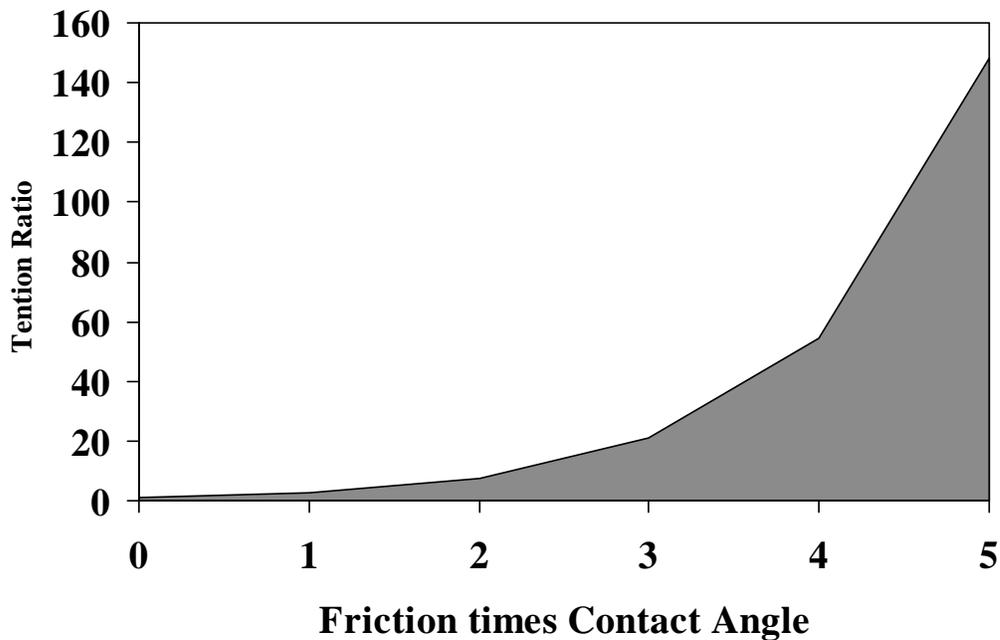
Figure 5: Example of exponential function of contact behavior.
