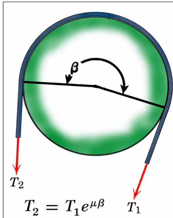
Figure 4: The capstan equation for belt friction.
